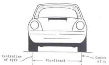
Wheel track is the distance measured across an axle from the centre line of one tyre tread to the centre line of the opposite tyre tread.
