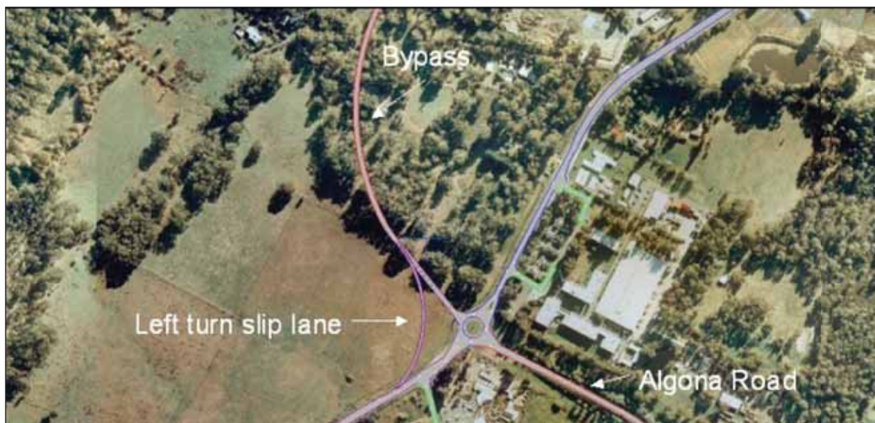
Figure 9 Bypass Option BP10 with Left Turn Slip lane at Algona Road
