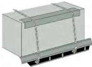
A correctly lashed and fastened load.
