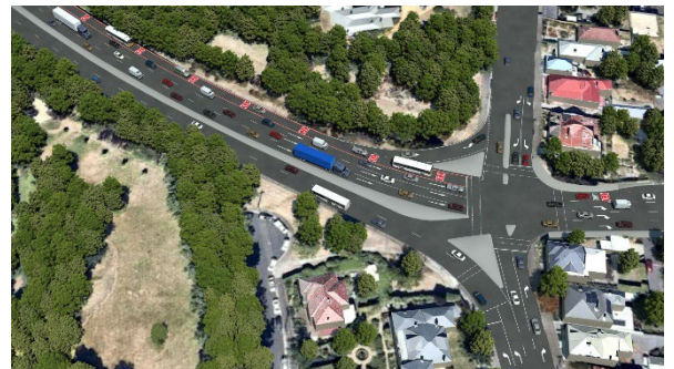
Image 1: Proposed Southern Outlet Transit Lane intersection depicting transit lane approach and realigned intersection, traffic islands and crossings.
