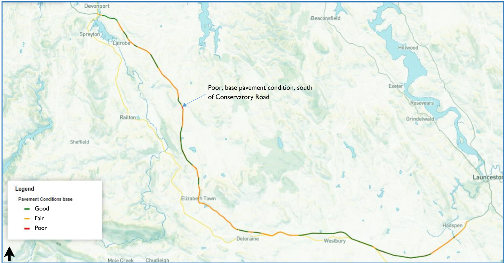
Figure 4.9: Base pavement condition
