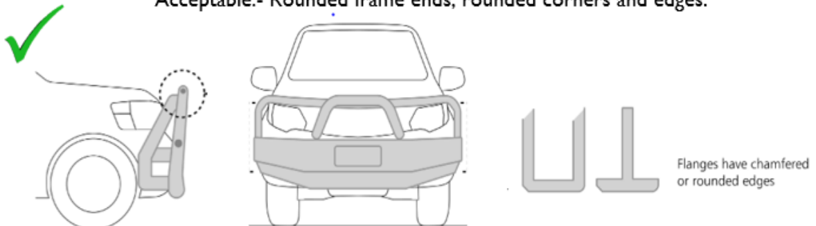
Acceptable:- Rounded frame ends, rounded corners and edges.
