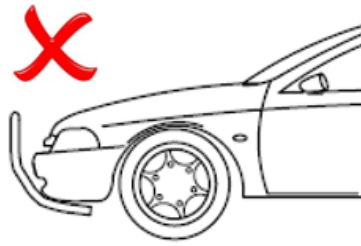
Unacceptable Offset "O" exceeds 75mm (greater than 9 degrees)
