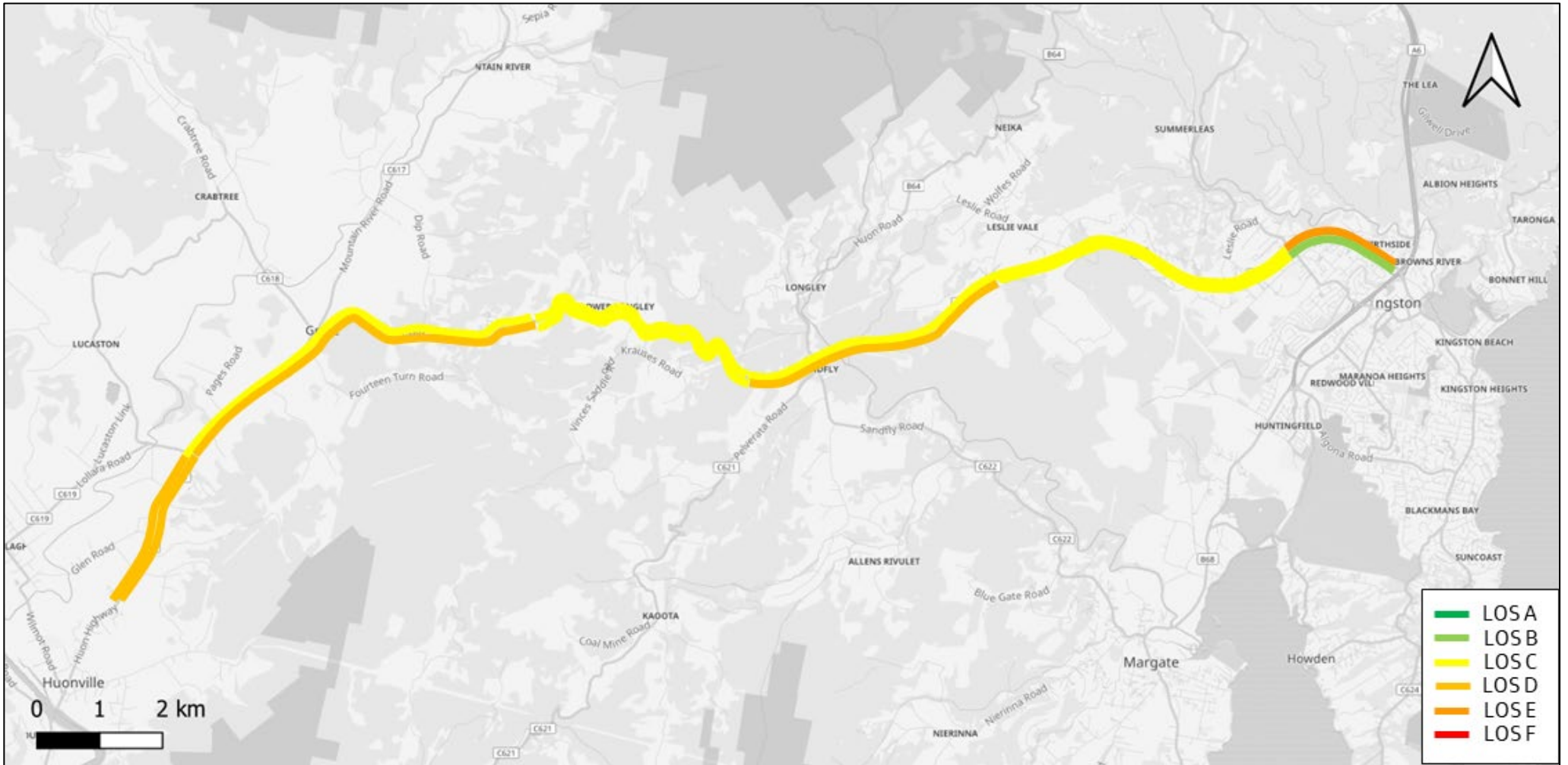
Figure 4-9: LoS along corridor
