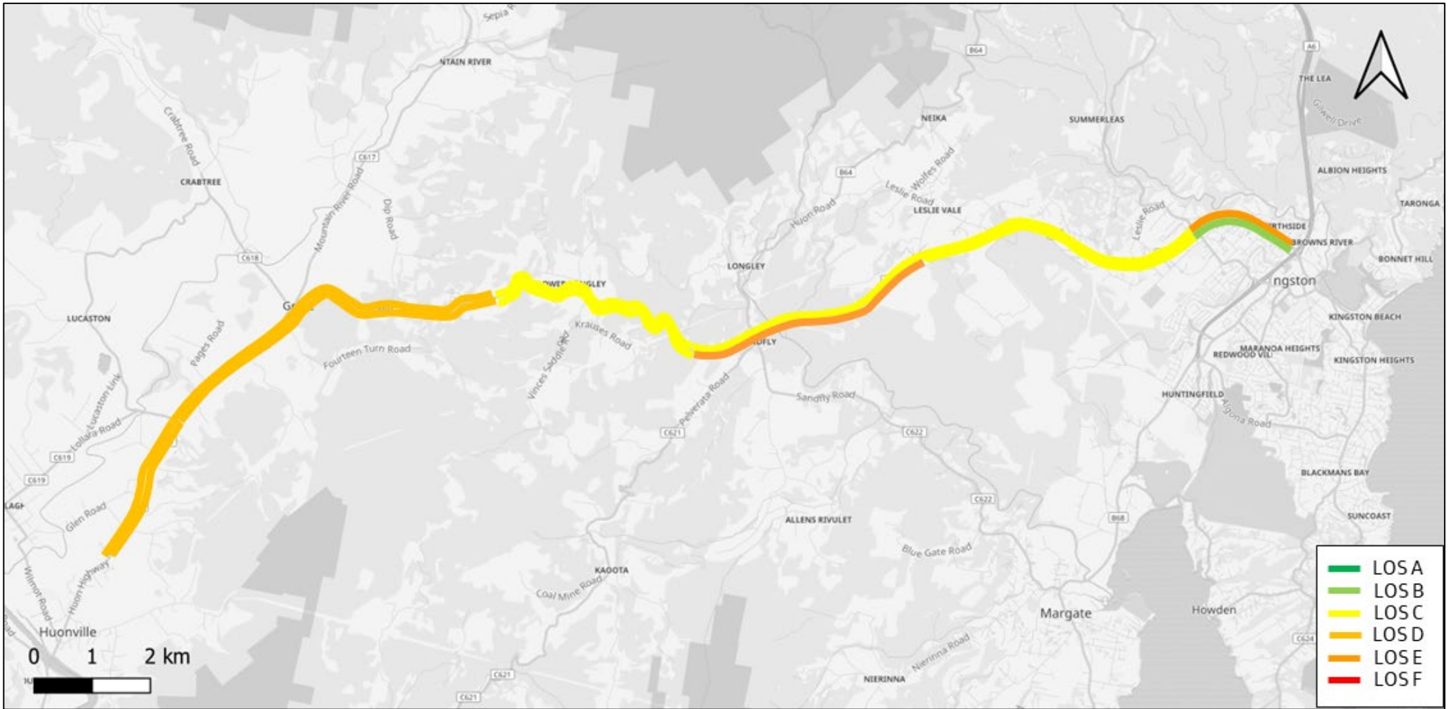
Figure 5-3: 2051 LoS along corridor (GHUTDM traffic volume projections)
